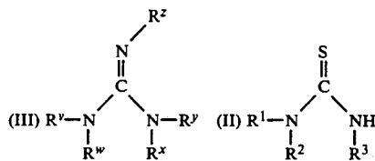
with  $H_2O_2$  and a molybdenum catalyst to yield an aminoiminomethane sulfonic acid which can then be reacted with an amine followed by optional transamination steps.
