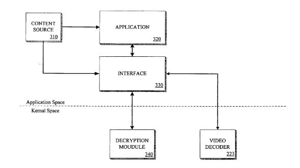
(57) Abstract: According to one embodiment, a method is disclosed. The method includes receiving video data at an application program, receiving the video data to one or more memory buffers, decrypting the video data, and monitoring page table entries corresponding to the memory buffers to determine whether a second application program has accessed the memory buffers.
