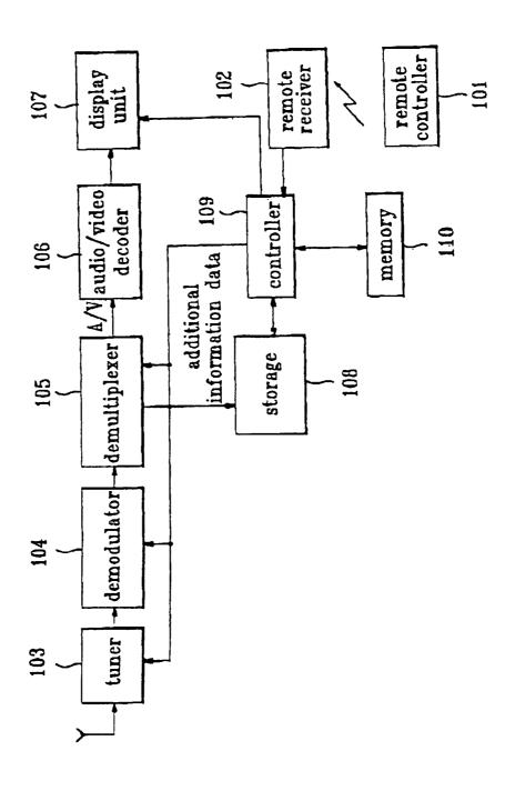
controller remote 102 remote reciver 101 display unit 107 audio/video controller 201 memory decoder 106 or detailed information information external detailed information data on each object demultiplexer decoder MODT modem 105 additional information data added demodulator 202 104 203 103 tuner +
