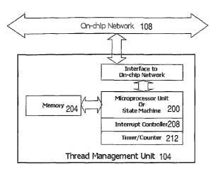
(57) Abstract: Methods and apparatus for dedicated thread management in a CMP having processing units, interface blocks, and function blocks interconnected by an on-chip network. In various embodiments, thread management occurs independent of any particular processing unit allowing for fast, low-latency switching of threads without incurring the overhead associated with a software-based thread-management thread.
