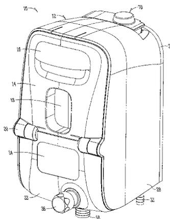
provide for one way flow and the prevention of backflow of a product chemistry into a water supply. The flow control may be selected based on the regulatory standards of the location used.
