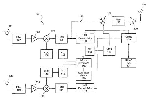
(57) Abstract: An AM/FM radio receiver is integrated with a wireless phone unit. Preferably, a wireless headset communicates with the integrated unit to selectively provide both commercial radio audio and wireless telephony. A microphone unit allows the user to conduct a wireless telephone call from the headset.
