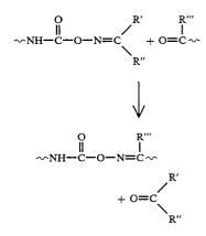
In this scheme, the crosslinking is effected by transoximation.
