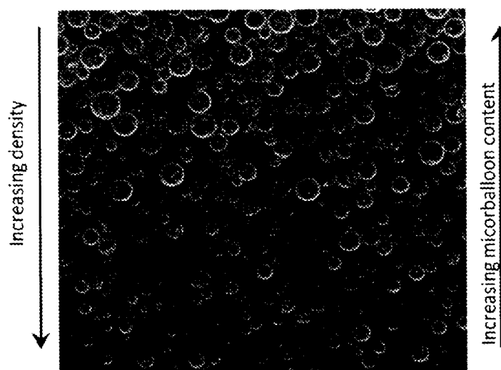
Research sample micrograph of microballons in resin matrix
