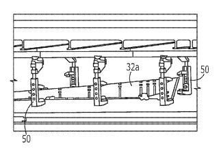
system includes a side of body cell configured to receive a spliced panel from the splicing cell and to attach a side of body chord thereto to produce a wing panel.
