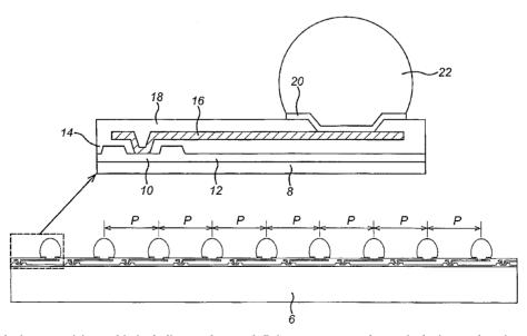
(57) Abstract: A device comprising a chip including a substrate defining one or more electronic devices and a printed circuit board electrically connected to the chip via one or more solder elements sandwiched between the chip and the printed circuit board, and the solder elements, said buffer layers having a Young's Modulus of 2.5GPa or less.
