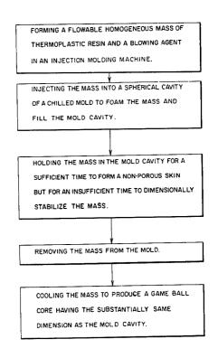
FORMING A FLOWABLE HOMOGENEOUS MASS OF THERMOPLASTIC RESIN AND A BLOWING AGENT IN AN INJECTION MOLDING MACHINE.
