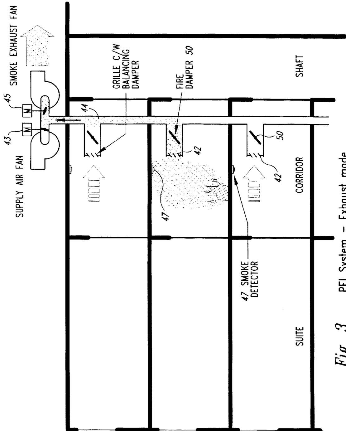
Fig. 3 PEI System - Exhaust mode
