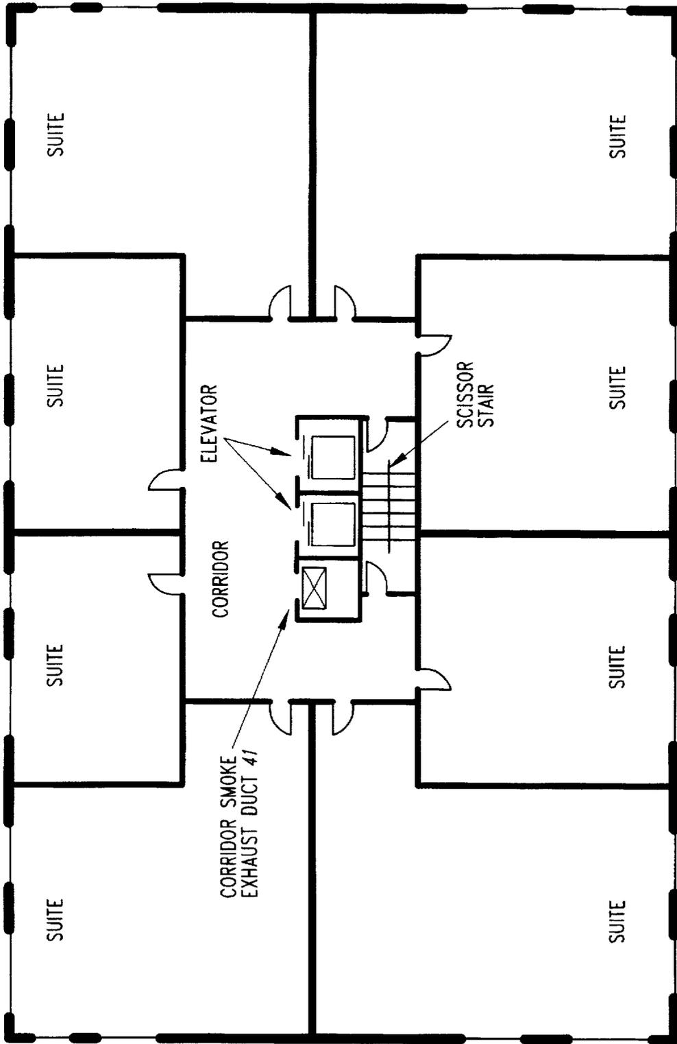
*Fig. 7* Typical central core floor plan
