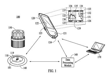
(57) Abstract: Devices, methods, systems, and kits for providing electronics for coupling to analyte sensors are provided including, for example, application specific integrated circuit (ASIC) architectures and configurations that provide electrical coupling of electrodes of analyte sensors having one or more configurations such as, for example, self powered two electrode analyte sensors, or three electrode analyte sensors.
