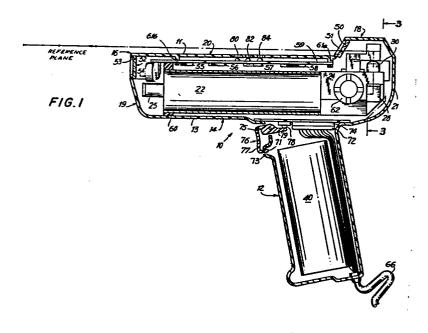
The present invention generally relates to laser scanning systems for scanning, reading and/or analyzing bar code symbols and, more particularly, to a light-weight, easy-to-manipulate, non-arm-and-wrist-fatiguing, hand-held, narrow-bodied, single-and twin-windowed, laser scanning head supportable entirely by a user throughout the reading of the symbols.
