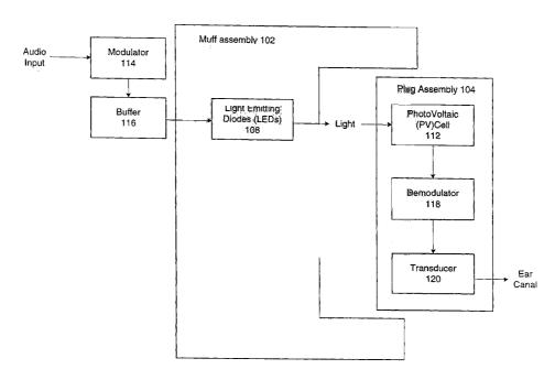
(57) Abstract: A hearing protector assembly has a muff and an ear-plug for hearing protection while allowing reception of audio communication. The muff has a receiver for audio signals, a modulation circuit, and a set of LEDs for transmitting the audio signal as a light signal. The ear-plug has a photovoltaic cell for receiving the light signals, a demodulator circuit, and a transducer for converting the received signal into an acoustic signal.
