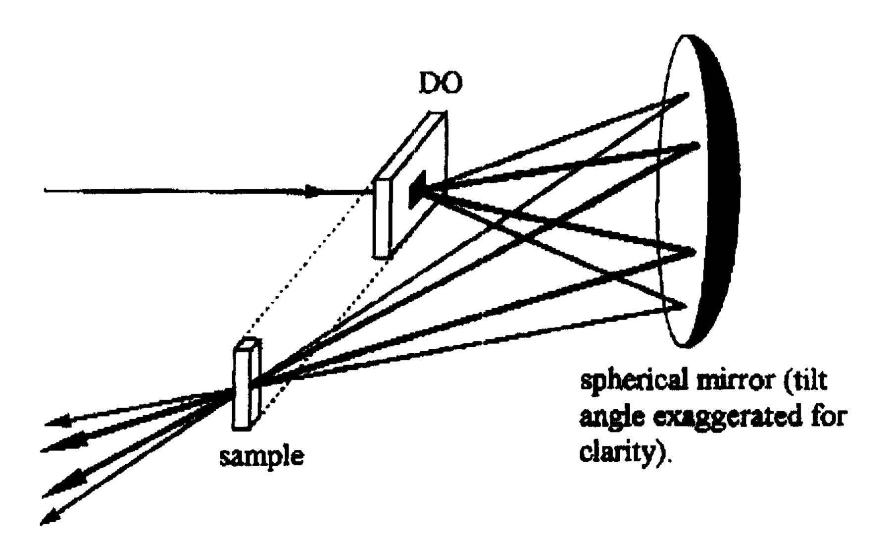
Fig. 2. Imaging setup for writing diffractive elements using a diffractive optic phase mask. Two different wavelength beams are shown: short wavelength = thick rays; longer wavelength = thin rays. Since the different colors are diffracted into different directions, the period of the structure written is independent of the source wavelength. This property is usually only obtained for near-field coupling of a phase mask into a sample.
