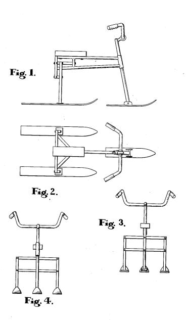
FIG. 1 is a side elevation view of my ski-cycle, showing my new design.
