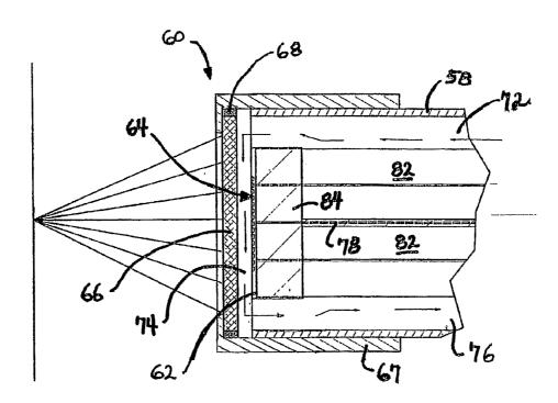
(57) Abstract: The present invention provides a thermal management system for semiconductor devices such as an LED array that applies a coolant directly to the LED array. Preferable, the coolant is an optically transparent cooling fluid that flows across the LED array and circulates through a system to remove heat generated by the LED array.
