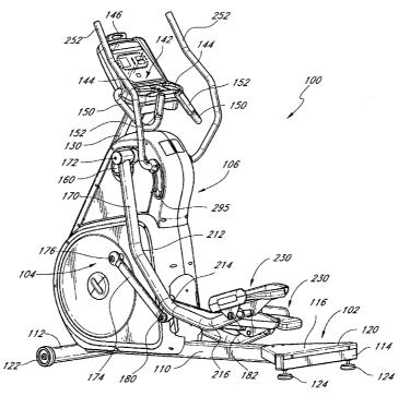
(57) Abstract: An elliptical machine has a frame and an operating linkage between the frame and foot supports. Each side of the operating linkage comprises five links that are connected with five pin joints. A foot support is connected to each side of the operating linkage with each of the five pin joints being positioned forward of the foot support.
