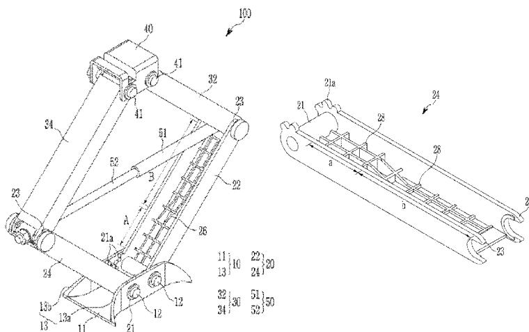
the lower arm and the upper arm and providing a tucking driving force to the lower arm and the upper arm. Herein, multiple reinforcing ribs are formed with different heights in a lengthwise direction of the lower arm and wherein the upper arm, the base portion, the lower arm, the upper arm, and the bracket member are made of a plastic material.
