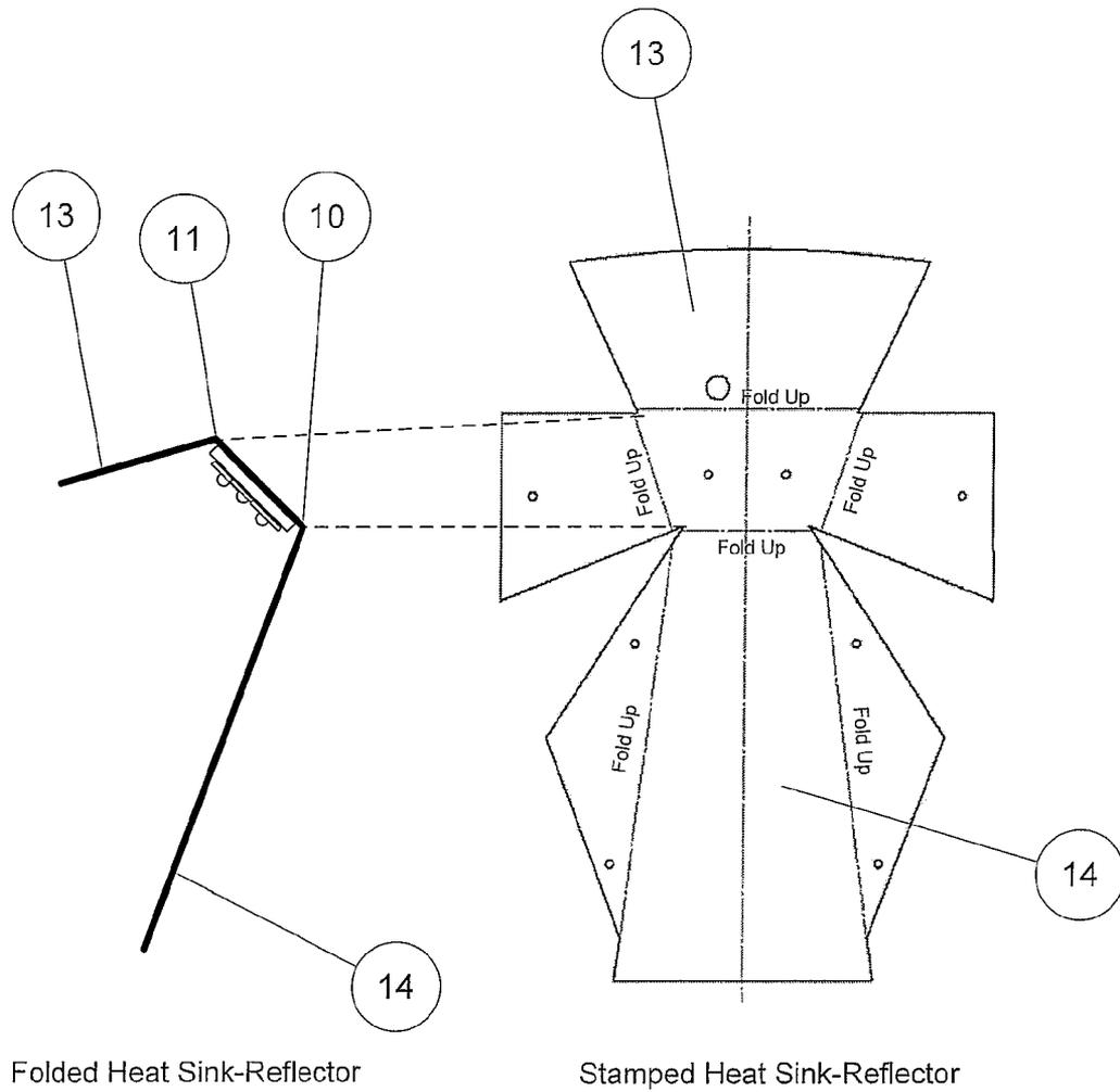
Figure 8 – Heat Sink-Reflector for Six Sided Fixture With Improved Directivity
