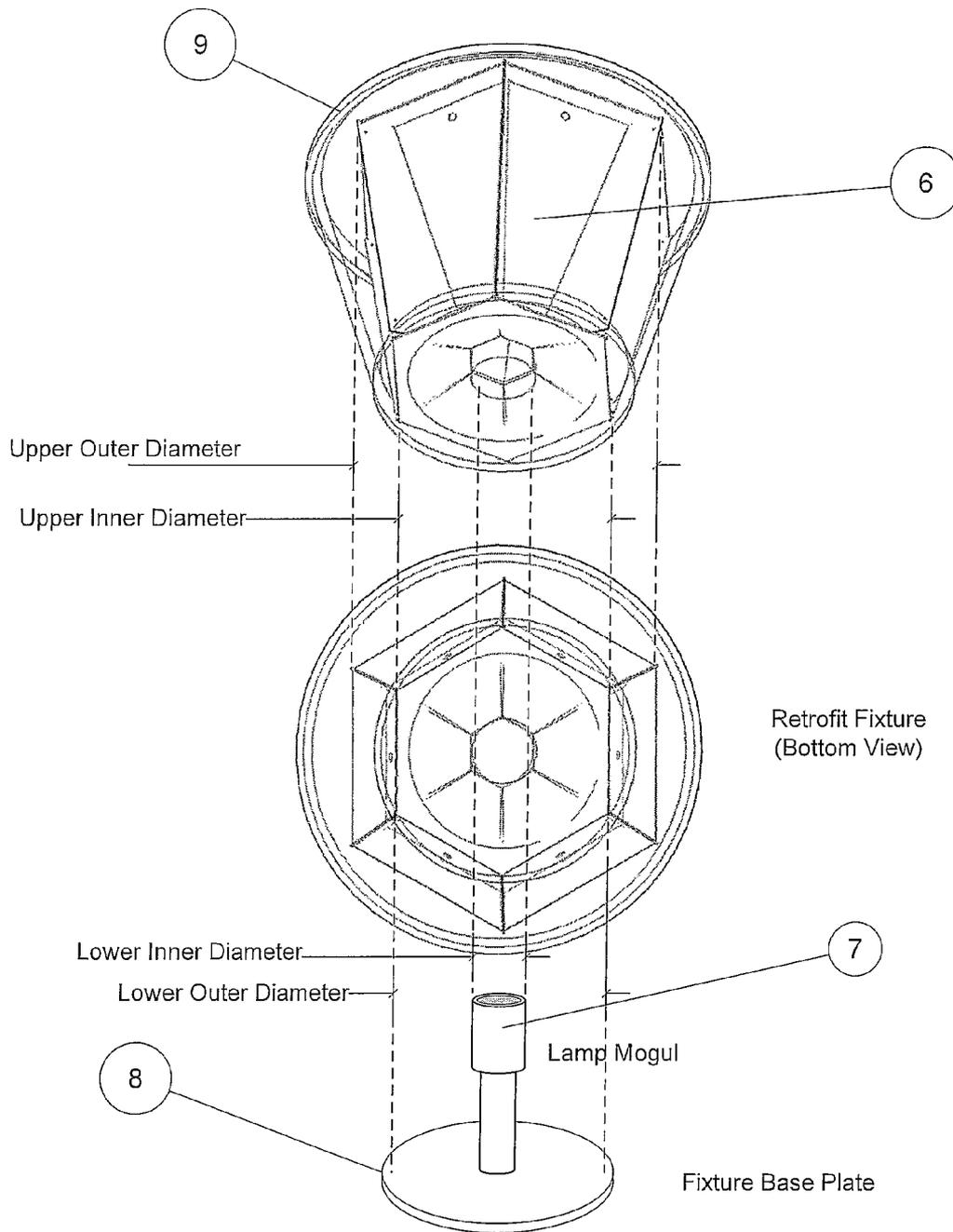
Figure 6 - Six Sided Led Fixture Assembly 16.7 Degree Tilt
