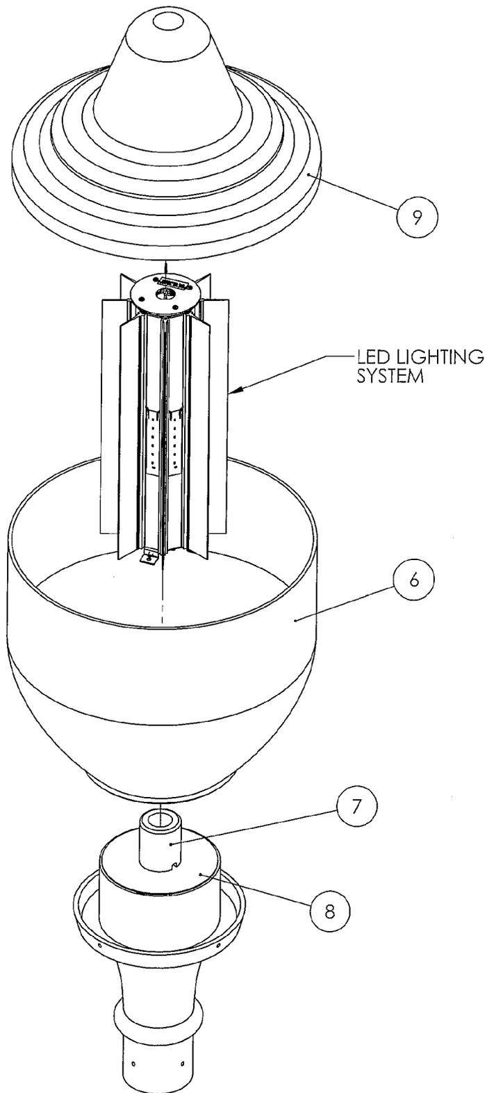
Figure 13: 8-Sided LED Fixture Assembly
