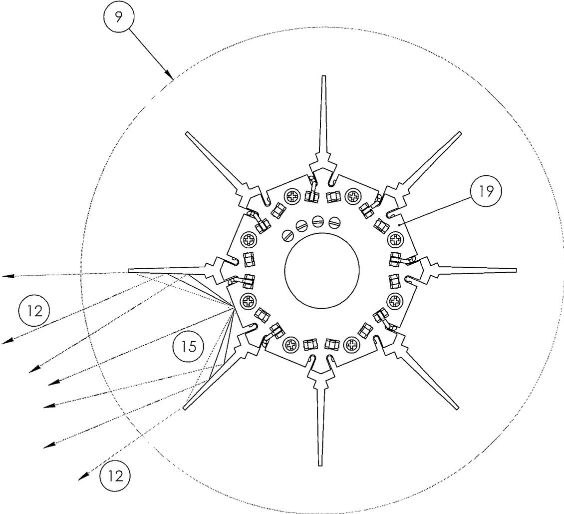
Figure 14: Sectional View Illustrating Light Ray Traces Between Fins
