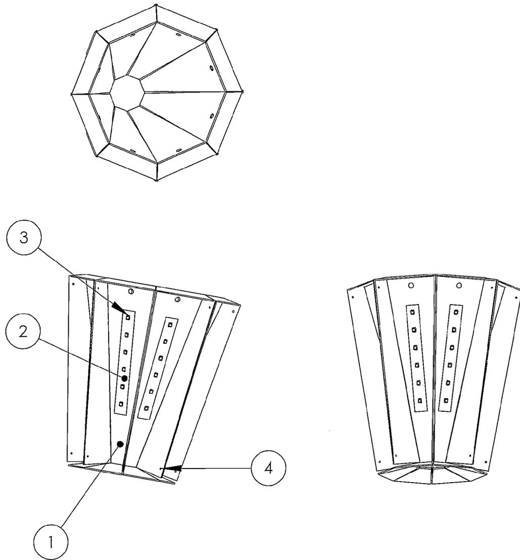
Figure 1 - 8-sided Led Fixture Assembly 16.7 degree tilt
