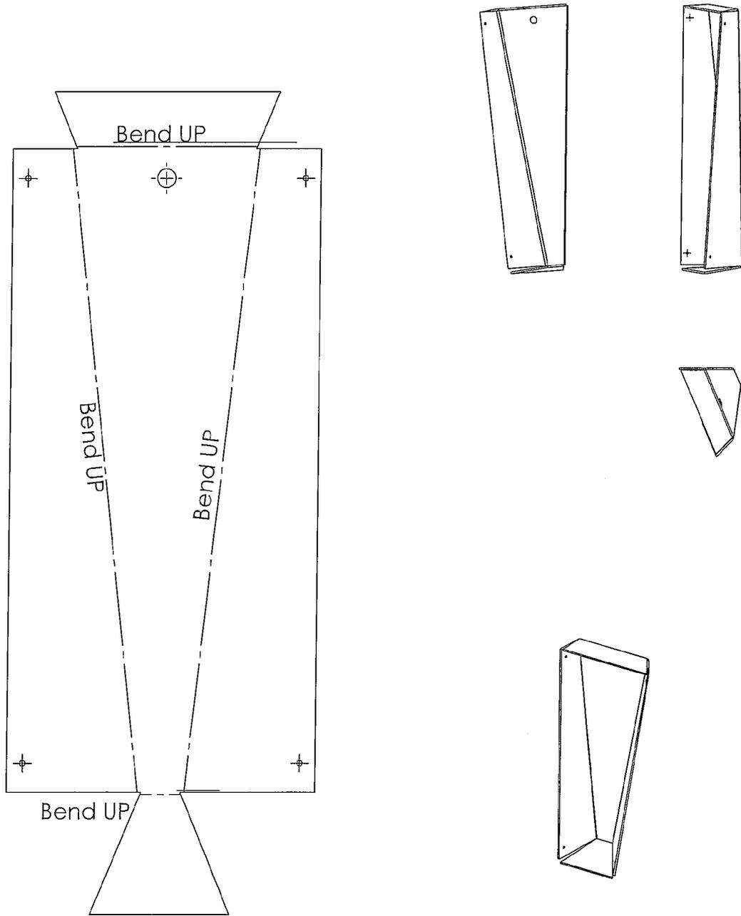
Figure 2 - Heatsink for 8 sided assembly - 16.7 degree tilt
