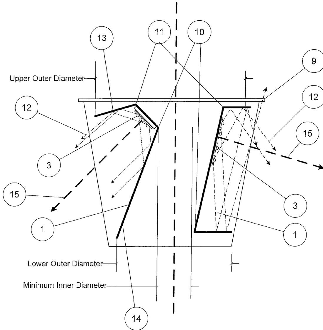
Figure 7 – Cross Sectional View Illustrating Light Ray Traces Comparison By Moving the Horizontal Fold Line
