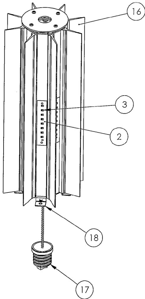
Figure 12: 8-Sided LED Fixture Assembly w/ Extruded Fins and Heat Sink
