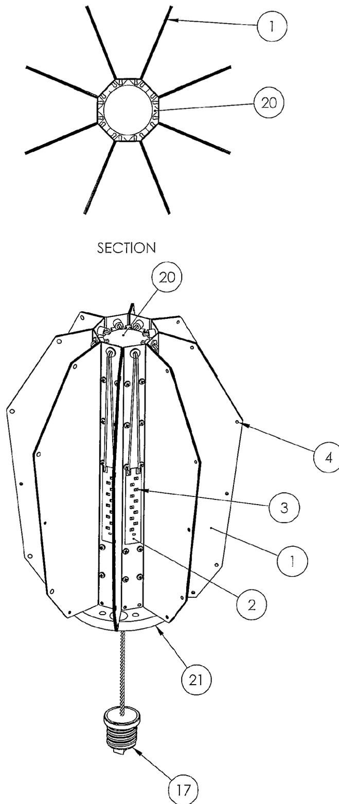
Figure 11: 8-Sided LED Fixture Assembly w/ Extruded Heat Sink
