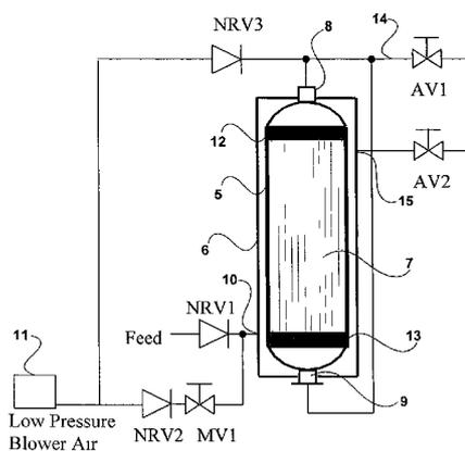
(57) **Abstract:** A method of backwashing a membrane filtration system comprising at least one permeable hollow membrane, the method comprising the step of applying a low-pressure gas to the permeate remaining present in the system when the filtration process is stopped or suspended to provide liquid for backwashing the pores of the membrane during a backwashing process.
