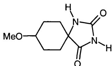
5      134.6 g [1.4 mol] of ammonium carbonate and 29.4 g [0.6 mol] of sodium cyanide are initially charged in 560 ml of water. Starting at room temperature, 38.5 g [0.3 mol] of 4-methoxy-cyclohexanone are added dropwise. The reaction mixture is stirred at 55-60°C for 16 hours, cooled to 0-5°C and stirred at this temperature for 2 hours. The solid is filtered off with suction and dried. This gives 57.88 g of a solid
