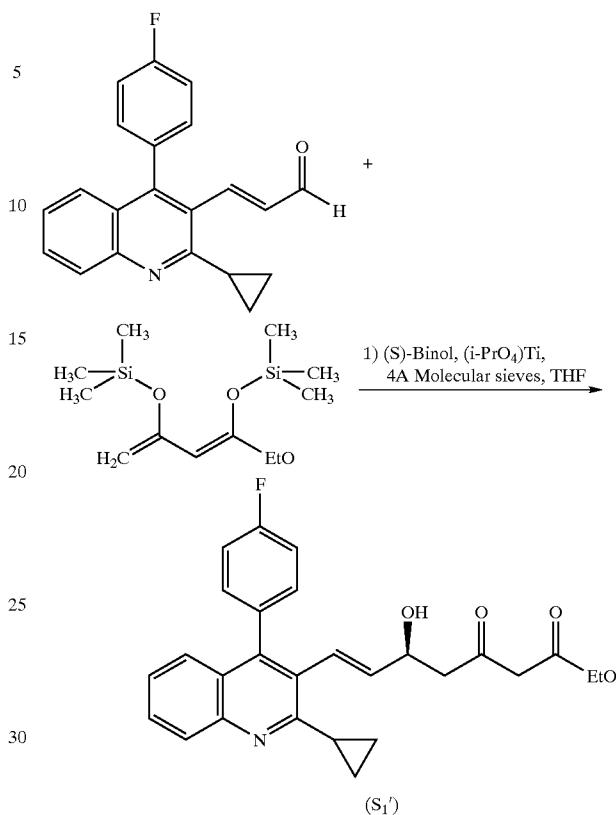
5(S)-hydroxy-3-ketoester (S<sub>1</sub>) was prepared using an external recycle reactor. The reactor contained a 0.5-L jacketed vessel equipped with a retreat-curve impeller and temperature sensor to determine the batch temperature; a recycle pump; a 1"-OD tube packed with solids; two three-way valves placed, respectively, at the inlet and exit of the tube; connecting tubing to form an external recycle loop; and a dosing pump for adding liquid to the recycle loop
