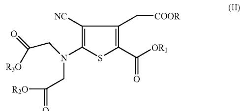
wherein R, R<sub>1</sub>, R<sub>2</sub>, and R<sub>3</sub> are independently a linear or branched C<sub>1</sub>-C<sub>6</sub> alkyl group or a substituted or unsubstituted C<sub>3</sub>-C<sub>12</sub> cyclic group, in the presence of a lithium base and in a solvent with an inorganic acid salt of strontium.
