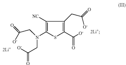
isolating the lithium salt of Formula III; and reacting the lithium salt of Formula III with the inorganic acid salt of strontium in a second solution to form the strontium ranelate or hydrate thereof.
