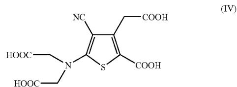
The acid of Formula IV is thereafter converted into its sodium salt and then converted into strontium ranelate using strontium hydroxide or strontium chloride in water.
