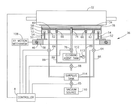
(57) Abstract: A service station (36) for servicing printheads, particularly inkjet printheads, which includes at least one blade-shaped wiper (78) and a plurality of pressure operated sprayers (74) fed with cleaning agents. The service station is subject to translational motion in both vertical and horizontal directions by an XY motion mechanism (108). In a method of employing the service station, the sprayers spray the cleaning agent onto the printhead prior to wiping.
