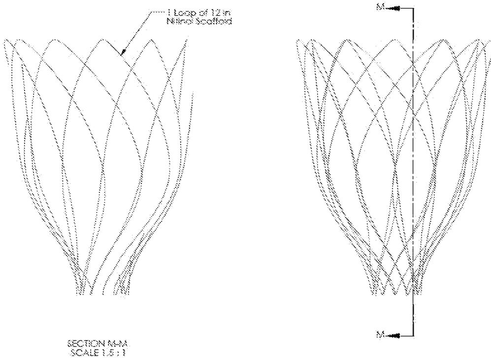
Nitinol Wire Scaffold: The right view shows the complete scaffold with 12 loops, the left view shows a section-view of the complete scaffold so the individual loops are more visible
