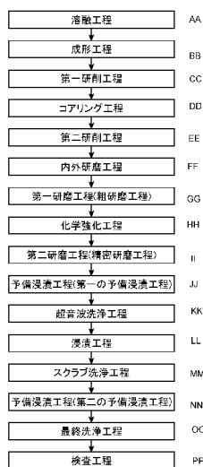
FIG. 1: AA Melting step BB Molding step CC First grinding step DD Coring step EE Second grinding step FF Internal/external polishing step GG First polishing step (lapping step) HH Chemical toughening step II Second polishing step (fine polishing step) JU Preliminary immersion step (First preliminary immersion step) KK Ultrasonic cleaning step LL Immersion step MM Scrub cleaning step NN Preliminary immersion step (Second preliminary immersion step) OO Final cleaning step PP Inspection step
