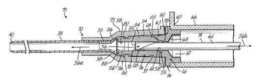
(57) Abstract: A generally rigid molded plastic catheter hub attachment (16, 52, 74) includes one or more co-molded elastomeric gaskets (22, 58).
