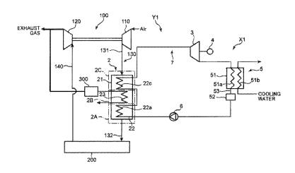
and an economizer, the heat exchanger including: a first heat section for heating a working medium by supercharged air from the supercharger; a second heat section for heating the supercharged air by steam generated by the economizer before the supercharged air flows into the first heat section; and a third heat section for heating the working medium having been heated in the first section by the supercharged air which is to be heated in the second section.
