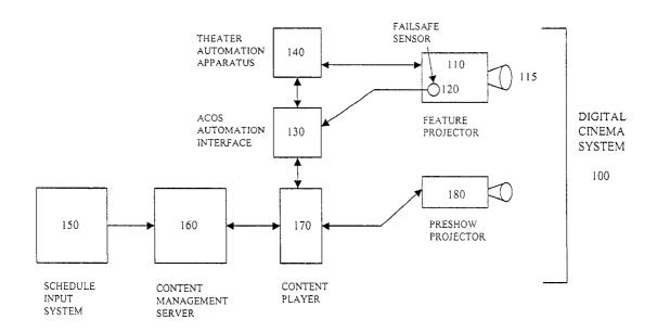
DIGITAL CINEMA SYSTEM 001 115 PRESHOW PROJECTOR FEATURE PROJECTOR 180  $\bigcirc$ 120 FAILSAFE SENSOR CONTENT PLAYER 170 140 130 THEATER AUTOMATION APPARATUS ACOS AUTOMATION INTERFACE CONTENT MANAGEMENT SERVER 160 SCHEDULE INPUT SYSTEM 150
