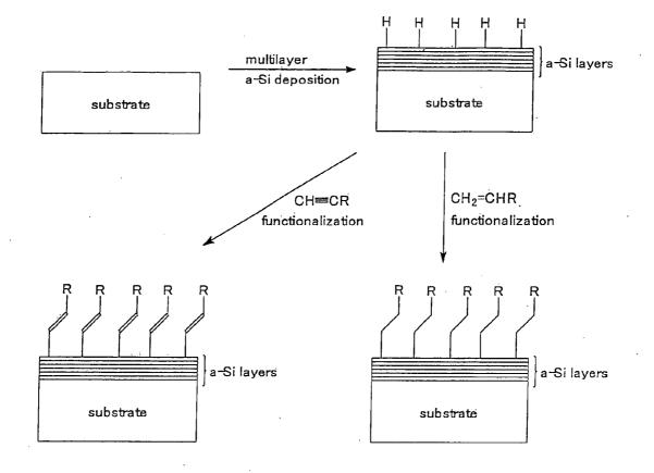
R = H, hydrocarbon, hydrocarbons, substituted hydrocarbons, carbonyls, carboxyls, esters, amines, amides, sulfonic acids, and epoxides
