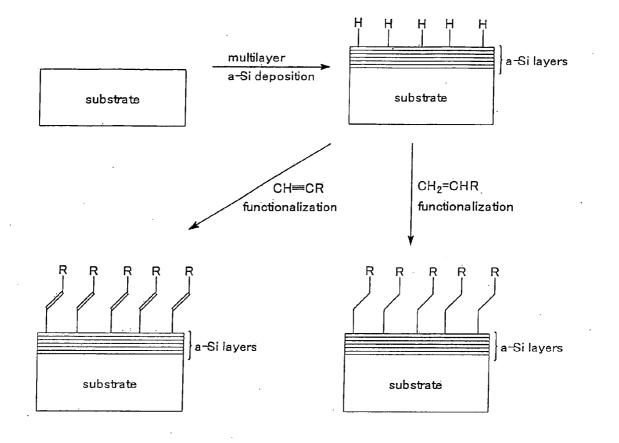
R = H, hydrocarbon, hydrocarbons, substituted hydrocarbons, carbonyls, carboxyls, esters, amines, amides, sulfonic acids, and epoxides
