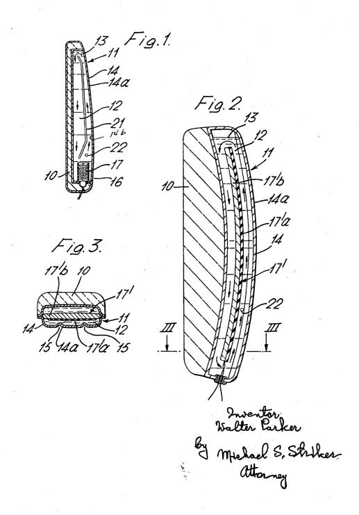
YARN HEATING MEANS IN TEXTILE APPARATUS
