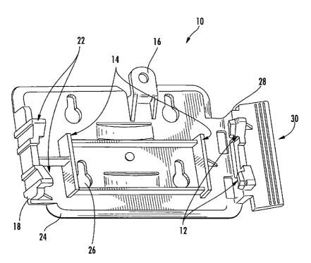
(57) Abstract: A mounting bracket may include a base plate, at least one stationary clip disposed on the base plate, a push releasing plate disposed in spaced apart relation to the at least one stationary clip, and at least one movable clip operatively coupled to and movable with the push releasing plate. The stationary clip or clips and movable clip or clips are disposed and configured to mate with cavities in respective ends of a pump when the push releasing plate is in a non-pivoted position
