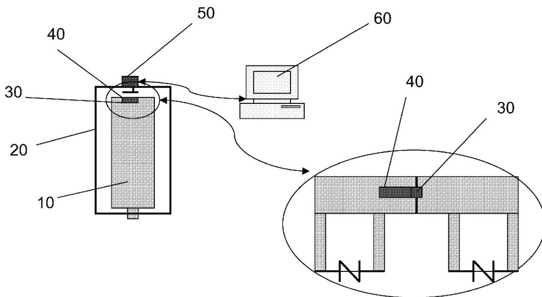
**Figure 2: Transmembrane Pressure Probe / RFID Communication Device within Multi-Element Filter Configuration**
