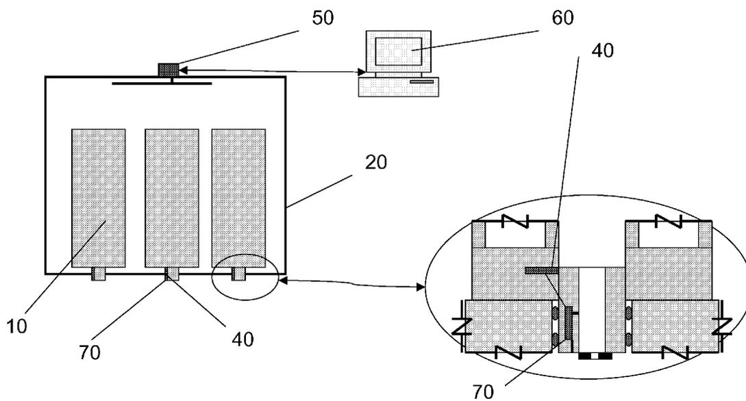
**Figure 5: In- Situ Integrity Test Configuration Pressure Sensor / RFID Communication Device within Multi-Element Tangential Flow Filter Configuration**
