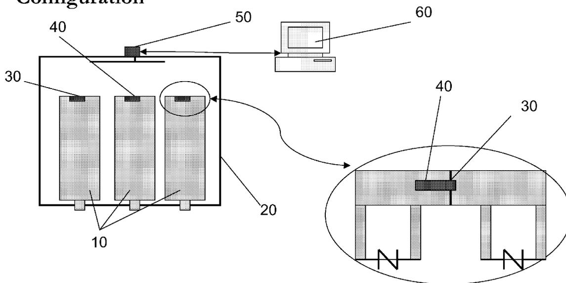
**Figure 3: In- Situ Integrity Test Configuration Transmembrane Pressure Probe / RFID Communication Device within Multi-Element Filter Configuration**
