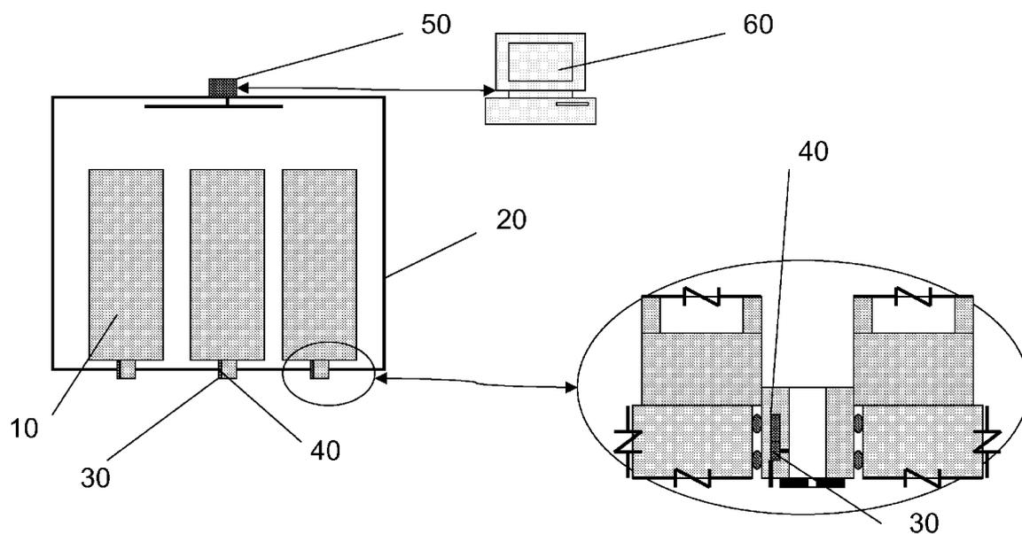
**Figure 4: In-Situ Integrity Test Configuration Flow Sensor / RFID Communication Device within Multi-Element Filter Configuration**
