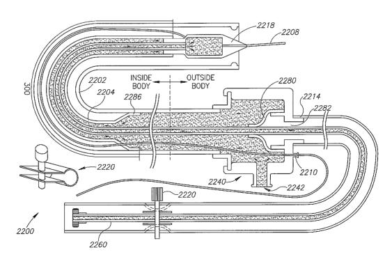
(57) Abstract: A catheter drive system, comprising: an inner tube adapted for inserting into a human body; an outer tube configured to slidably and snugly engage said inner tube, outside of a human body; and a pushing mechanism adapted to apply a pushing force to said inner tube less than 100 mm from an end thereof, such that said inner tube can extend at least 200 mm.
