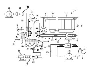
channel via a secondary combustion air nozzle provided on the combustion gas channel, in which the recirculated exhaust gas nozzle and the secondary combustion air nozzle are arranged in different positions in a plan view.
