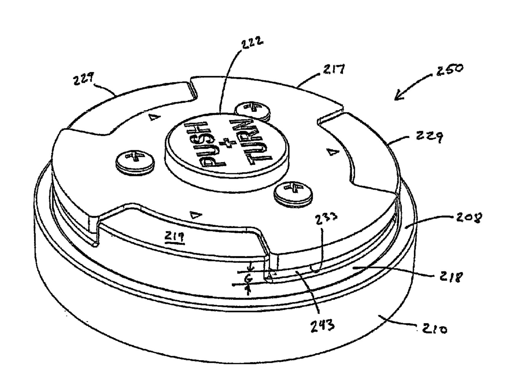
(57) Abstract: Aerodynamic wheel covers may include a hub assembly coupled with a hub of a large vehicle, such as a truck. A base assembly may be coupled to the hub assembly, and a disk assembly may be coupled with the base assembly such that removal and installation of the disk assembly may be accomplished without tools.
