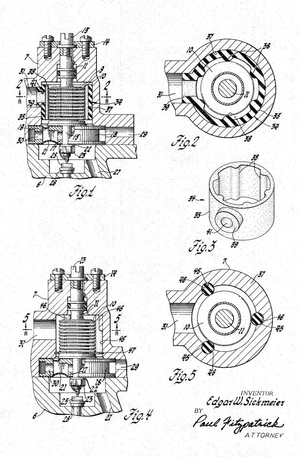
My invention relates in one aspect to means for damping vibrations of elastic bodies and in another aspect to means for increasing the reliability of elastic bellows in environments which vibration of such bellows is likely to be induced.
