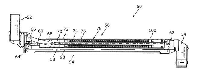
position of the mounting (68,70) of the lever arm (60) on the supporting arm (58) is adjustable along a longitudinal extension of the supporting arm (58). Further, the invention relates to a support arm system and a method for operating a support arm articulation device.
