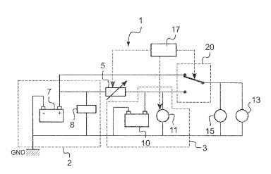
between the first (2) and second (3) circuits, said connecting member (5) allowing, in a first configuration, an exchange of current of a first value between the first circuit (2) and the second circuit (3) and, in a second configuration, an exchange of current of a second value between the first circuit (2) and the second circuit (3), in which the second value is lower than the first value; and a control unit (17) which controls the configuration of the connecting member (5).
