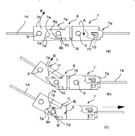
moves the two or more connecting parts toward or away from each other to open or constrict the angle of the joint around the longitudinal axis and/or the angle thereof around an axis orthogonal to the longitudinal axis, thereby disposing the treatment part at the desired position and in the desired orientation within the body cavity.
