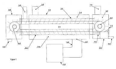
(57) Abstract: The present invention relates to a carbonization reactor (1-0) to decompose used rubber products and the like by heating the rubber products under constant high temperature and the reactor comprise a conveyor (2-0) which continuously move and drag the rubber products through cylinders (2-1, 2-2) where the decomposition process takes place to produce recyclable by products such as carbon black, oil vapour and the like.
