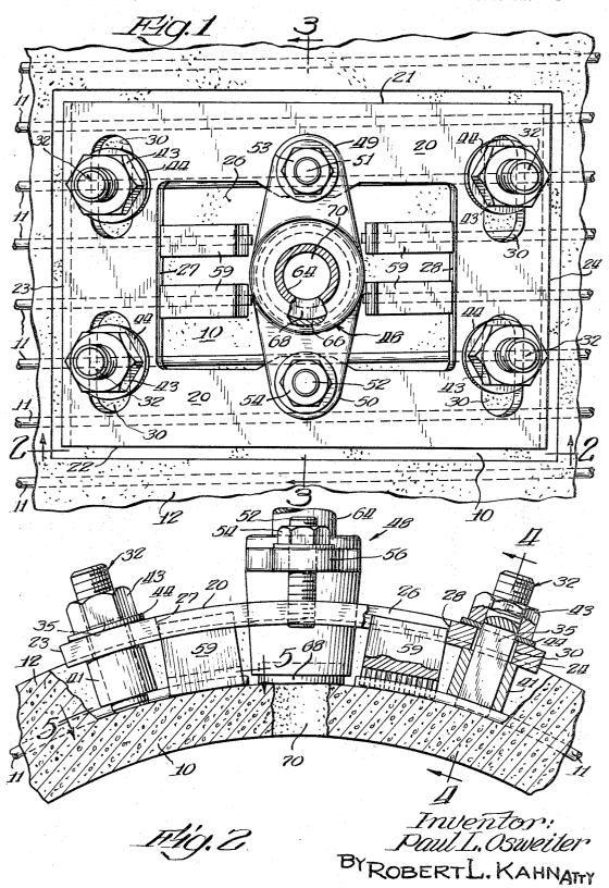
TAPPING SADDLE FOR PRESTRESSED CONCRETE PIPE
