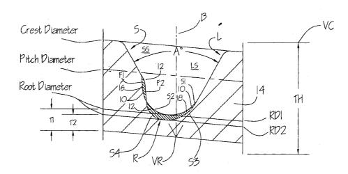
(57) Abstract: A thread form having improved strength and fatigue resistance. The root of the thread is cut on multiple cutting radii having displaced centers. At least two of the root surfaces are formed by cutting radii having lengths that are greater than the root truncation. The threads are used in a double start configuration to increase the connection strength and reduce makeup and breakout rotations
