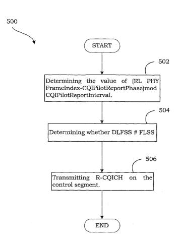
(57) Abstract: A method and apparatus for reporting CQI in a wireless communication system, the method comprising determining the value of (RL PHYFrame Index- CQIPilotReportPhase)mod CQIPilotReportInterval, determining if DLFSS is not equal to FLSS and transmitting R-CQICH on the Control segment.
