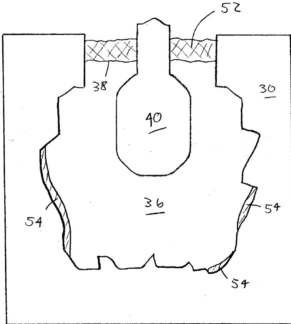
**DRILL BIT BODY WITH MULTIPLE BINDERS****CROSS-REFERENCE TO RELATED APPLICATIONS**
