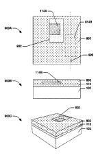
HM region, and a spacer region is deposited above the patterned PR and second sacrificial HM region. In some embodiments, at least some of at least one of the spacer region, the PR, or the respective sacrificial HMs is removed. In this way, a line end space structure associated with an end-to-end space is formed.
