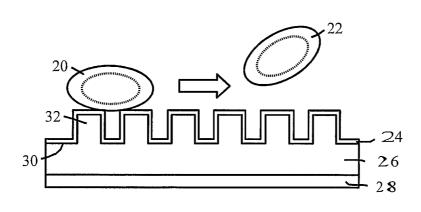
(57) Abstract: The present invention includes surface a (30) being formed of a synthetic polymer film (26) having pillars or ridges (32). The width, height, and spacing of the pillars or ridges (32) is such that platelets (20) will not adhere to the surface (30) to the extent that such would occur to a flat surface (18) even after a thin protein coating (24) has been deposited by the blood due to the reduced effective surface area of the surface (30).
