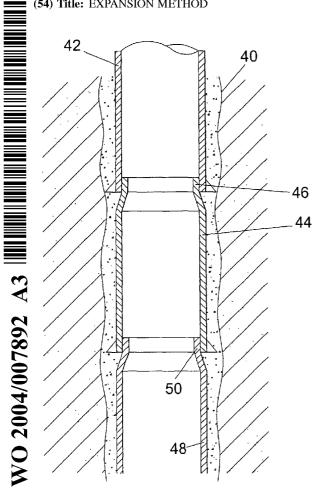
(57) Abstract: A method of expanding tubing downhole comprises the steps of: providing tubing (14; 44) of a first diameter; running the tubing into a bore (10; 40); expanding a first section of the tubing to a second diameter, and expanding a second section of the tubing to a third diameter.
